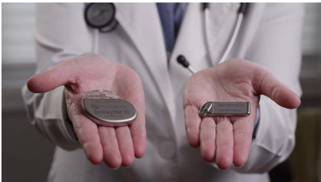
**Figure 2 - Axonics r-SNM™ implantable pulse generator (A) and patient therapy controller (B).**
